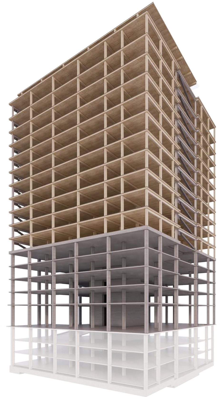
HYBRID MASS TIMBER TOWER
